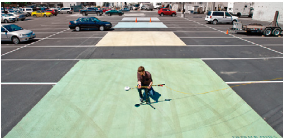
Lawrence Berkeley National Laboratory's cool pavement showcase, US Department of Energy Image Source: Landscape Architecture Magazine
