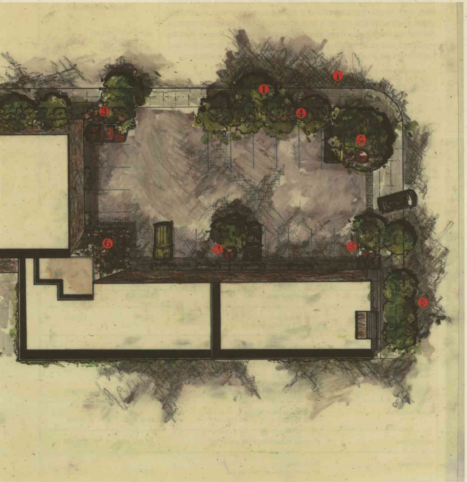
The design team's illustrative site plan shows the location of the various BMPs. They include increasing shade (1), underground cisterns (2), roof water cisterns (3), infiltration chimneys (4), off-site infiltration zone (5), and green roofs (6).
