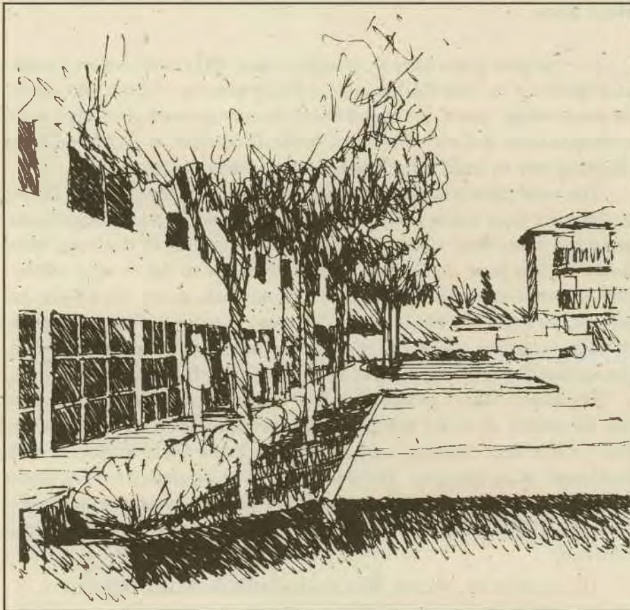
A mulch and grass filter bed separates the parking area from the buildings and provides a shaded green edge.
