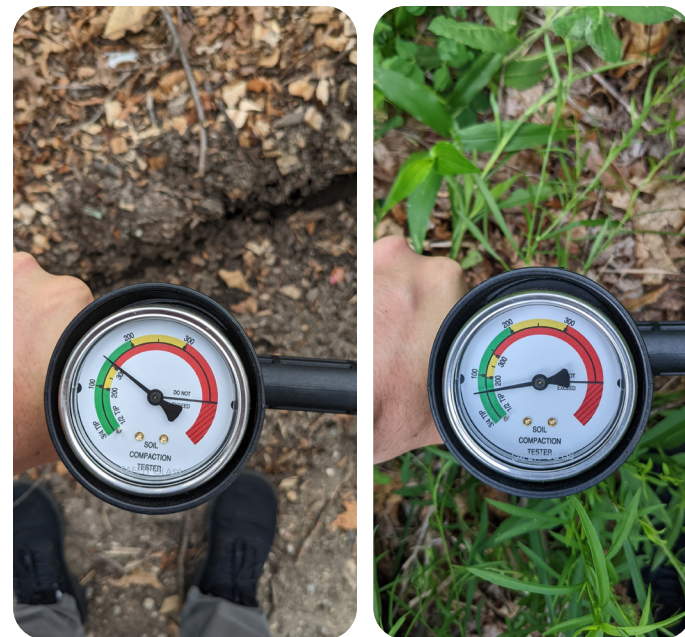
Figure 9. Monitoring changes in soil compaction at the demonstration project was key to communicating BMP effectiveness. Here a soil penetrometer is used to measure compaction: un-rehabilitated site (left) vs rehabilitated site (right). (photos: Vincent Verweij)
